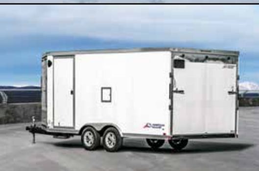
Mid-Deck design provides higher ground clearance for snow and off-road terrain
